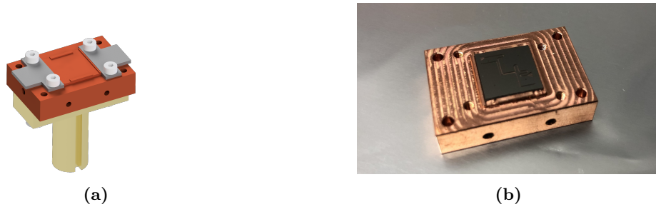
Figure 6.2: Images of the designed sample holder. (a) shows a CAD drawing of the sample holder, that is attached to the sample holder of the cryostat. On its top side, left and right of the centre chip platform, flexible printed circuit boards will be attached, which is schematically shown here. In (b), photograph of the built sample holder is shown. It also includes an early-stage fabrication test chip that is placed on the chip platform, where it will be attached to permanently later on.
