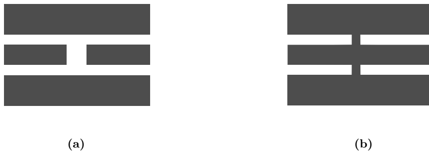
Figure 3.2: Coplanar waveguides in top view, with inserted impedance discontinuities. In (a) an open end in the waveguide is shown, which forms a capacitive discontinuity. In (b) a short end is illustrated, which introduces an inductive impedance mismatch.
