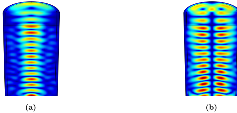
Figure 5.5: Possible eigenmodes of a cylindrical bulk acoustic resonator consisting of a high-quality acoustic substrate with a piezoelectric layer on top, as a result of an eigenfrequency study in Comsol. (a) to (b) show the three-dimensional surface displacement of the resonator for different modes.
