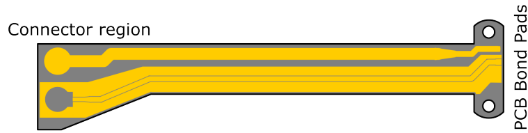
Figure 6.3: Layout of one flexible PCB for powering the atom chip. It contains one direct current line (top structure) to feed the on-chip trapping wire and a coplanar waveguide (bottom structure) for the connection to the on-chip coplanar waveguide resonator. Both lines will be connected to cables in the connector region and to the chip via the PCB bond pads. In the connector region of the PCB, the SMP footprint for soldering the SMP connector to the PCB can be seen in the bottom.
